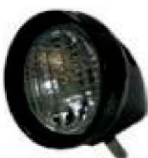
00801-BK & 00801-WH : Deck Spot Light & Spreader Spotlight Made of strong PVC, SS Parts, 12V 35W Halogen Beam (4-1/2").
