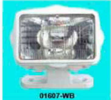
01607-WB : Roll-Bar Spot Light 12V 60W, ABS Housing for Vertical adjustment. 180mm x 120mm ( Housing Dia.) 160mm x 100mm ( Beam Dia. ) 165mm x 45mm ( Base Dia. ) 8mm Screw Holes.
