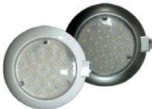
J-689-LED Switches waterproof IP66 Plastic PC base O.D. 150 mm. Plastic PC lens Dia. 120 mm. 21 super bright LEDs. Standard 21 LEDs. SPECIAL OPTIONS: with 30-white-LEDs. with 21-white plus 9 red ( or blue ) LEDs. color available -white and silver grey.
