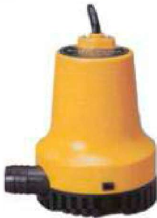
TMC-03603 TMC-03603 : 1850 GPH BILGE PUMP POWER SOURCE : DC 12V / 24V OUTLET DIA. : 1 1/8" CURRENT : 10A ( 12V ) , 5A ( 24V ) Delivery Head : 13.5FT ( 4.1M )
